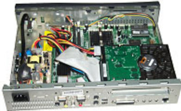
Hard Drive Mounted In Place (Rear View)
