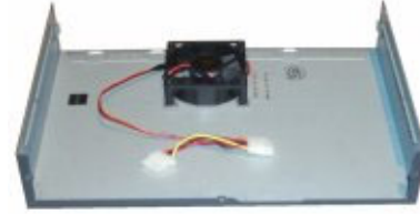
Fan Mounted to Enclosure Cover
